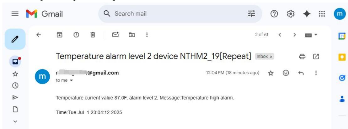
Tip: If the alarm description contains the **current value and enter alarm level 1/2/3**, it indicates that the alarm state is triggered, and only the **current value** contains the repeated alarm information.
